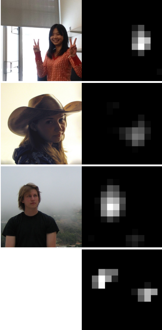
Figure 2. A view of the 13 \times 13 activations of the 151 st channel on the conv5 layer of a deep neural network trained on ImageNet, a dataset that does not contain a face class, but does contain many images with faces. The channel responds to human and animal faces and is robust to changes in scale, pose, lighting, and context, which can be discerned by a user by actively changing the scene in front of a webcam or by loading static images (e.g. of the lions) and seeing the corresponding response of the unit. Photo of lions via Flickr user arnolouise, licensed under CC BY-NC-SA 2.0.
